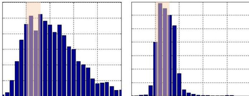
Fig. 4: Distribution of the fines flow; Operator + Old measurement (left) & APC + New measurement (right) - Improved process quality by reducing variation in fines (with quality range marked).
