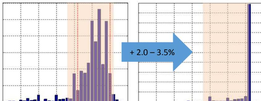
Fig. 5: Distribution of the production quantities; Operator (left) & APC (right) - Increased granulation production by pushing continuously to production limit (with production range marked).
