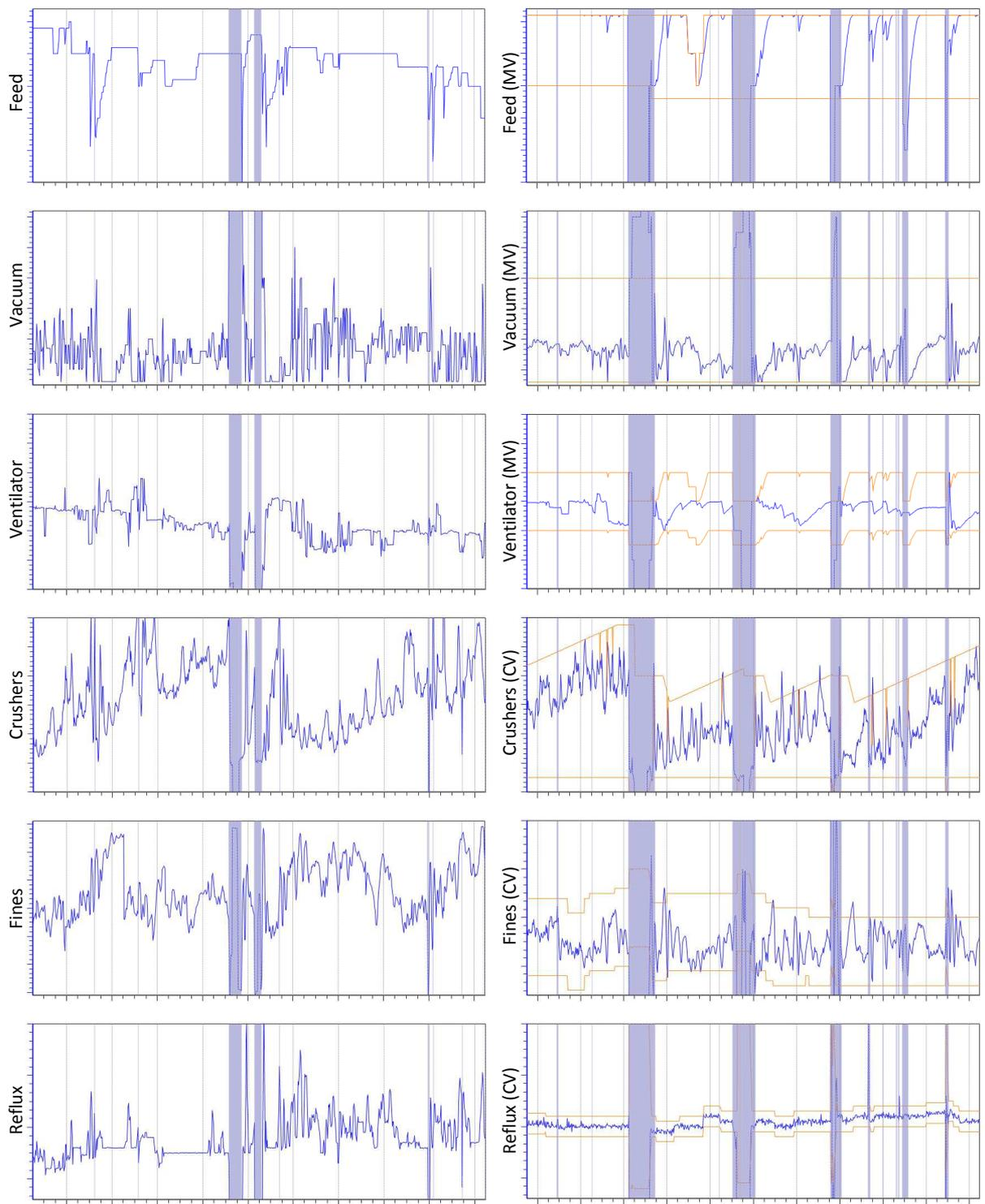
Fig. 2: Granulation operation (3 weeks); Operator (left) & APC (right) – Maintenance/short stops and APC off marked; APC lower/upper limits orange.
