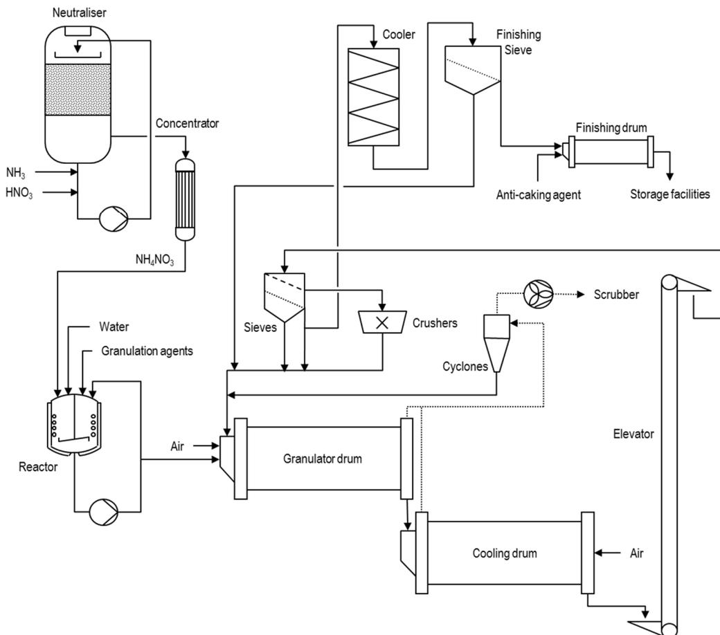
Fig. 1: Schematic overview of the granulation process.
