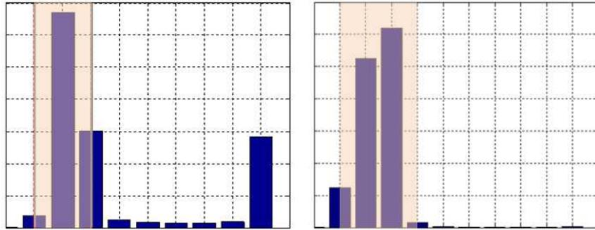
Fig. 3: Distribution of the reflux valve; PID (left) & APC (right) - Improved process stability by keeping reflux valve in control (with typical operating range marked).
