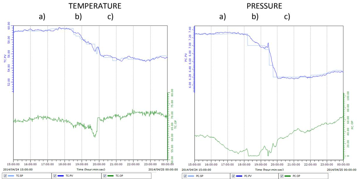
Figure 7 – DIB top section control performance after “Aptituning” during condensers maneuver
