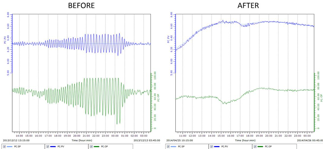
Figure 5 – DIB top pressure control: before and after “Aptituning” it
