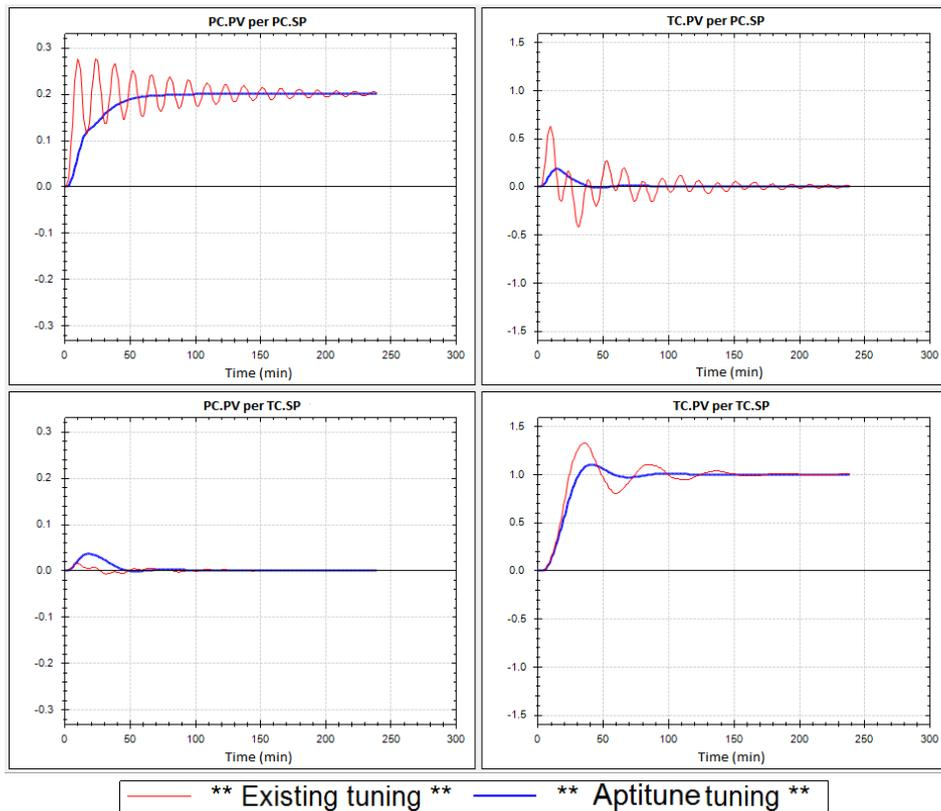
Figure 3 – 2x2 simulated typical step test response
