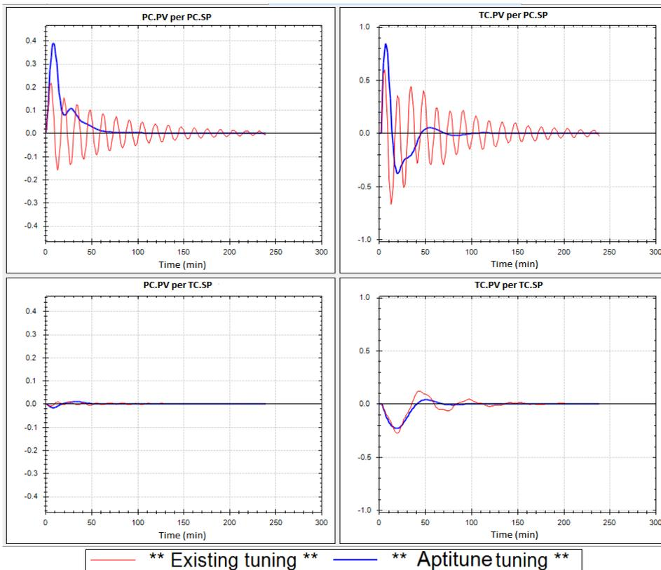
Figure 4 – 2x2 simulated typical load disturbance response
