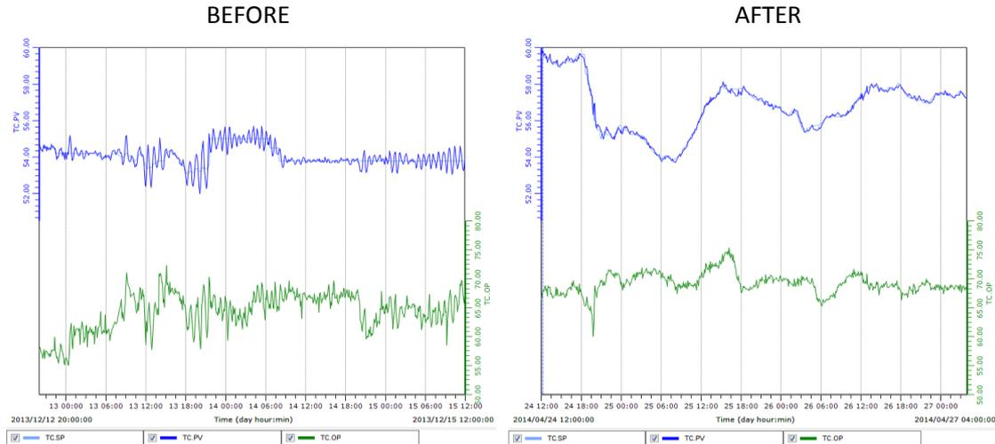
Figure 5 – DIB top temperature control: before and after “Aptituning” it
