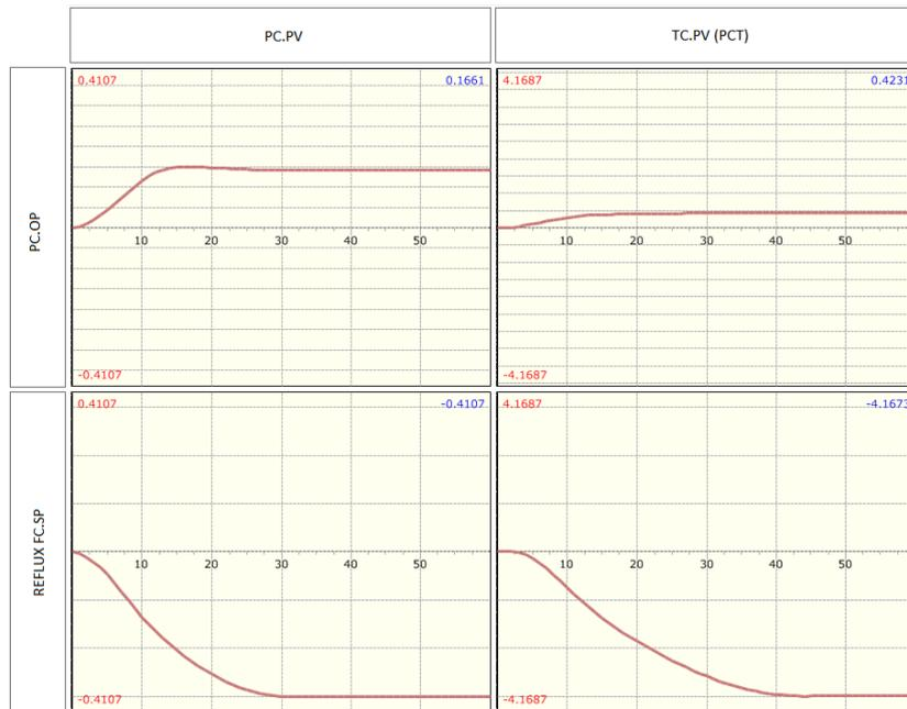
Figure 2 – Open loop step test models – scaled to independents typical steps
