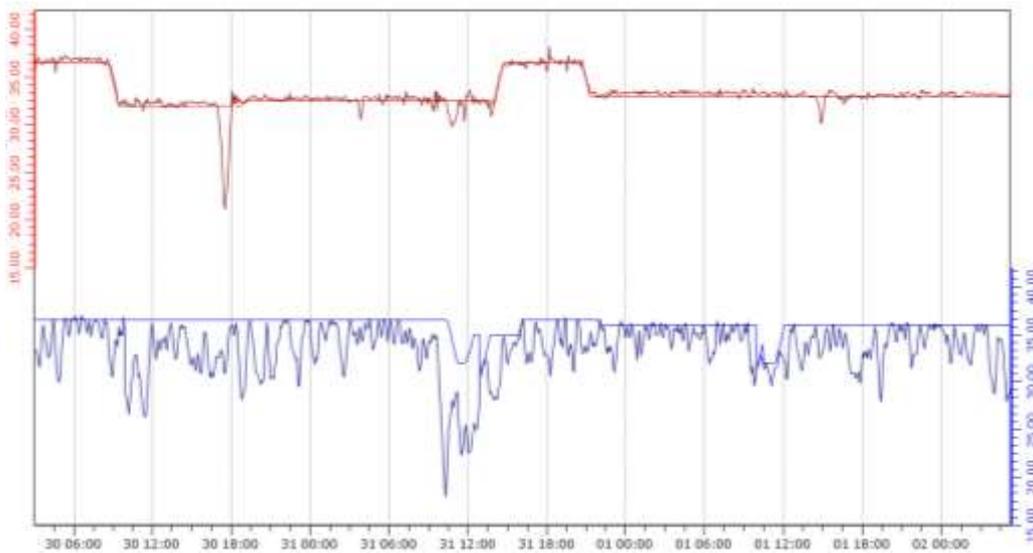
Figure 3 – Steam production after IPCOS assessment on waste incinerator (red) vs. identical boiler not yet assessed (blue)
