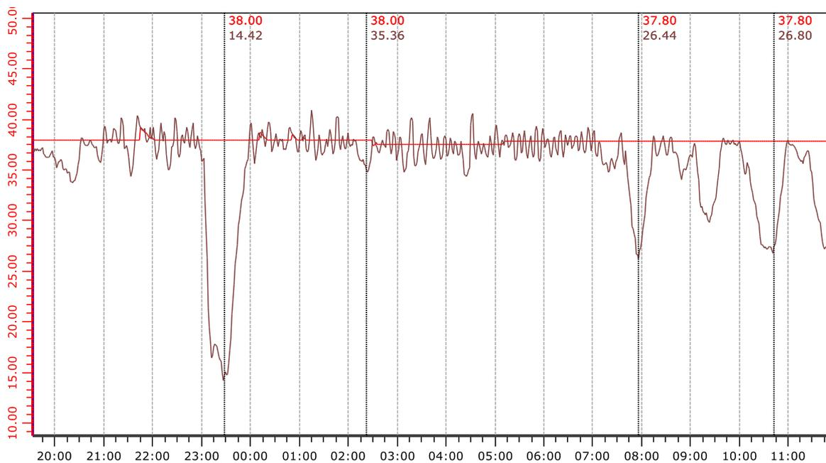
Figure 2 – Typical steam production variation on a waste incinerator boiler compared to the steam flow set-point
