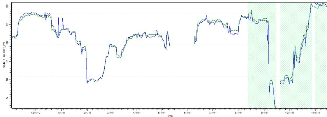
Figure 7: INCA Sensor: Process data (blue) versus Model Prediction (green).
