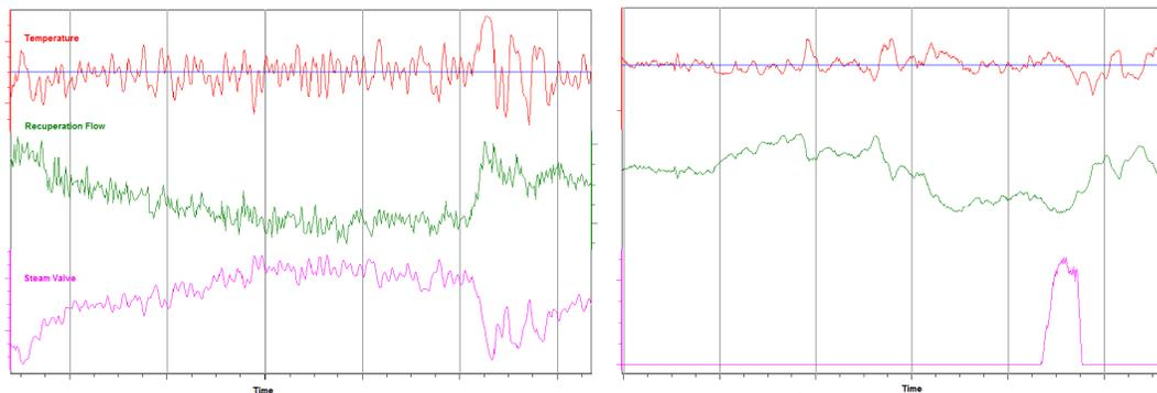
Figure 5: Performance of heat recuperation structure. Red: Temperature. Blue: Temperature Setpoint. Green: Recuperation flow. Pink: Steam valve position. Left: old control structure. Right: new control structure.
