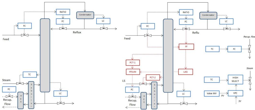
Figure 4. Left: Original control scheme. Right: Proposed control scheme that better fits the control objectives. New blocks are shown in red. The safety structure is conceptually shown by the six blocks on the right.
