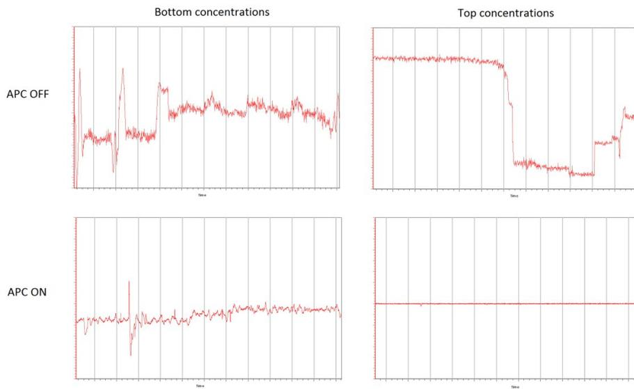
Figure 9: Bottom (left) and top concentration (right) trends over time. Upper plots: APC is turned off. Bottom plots: APC is turned on.
