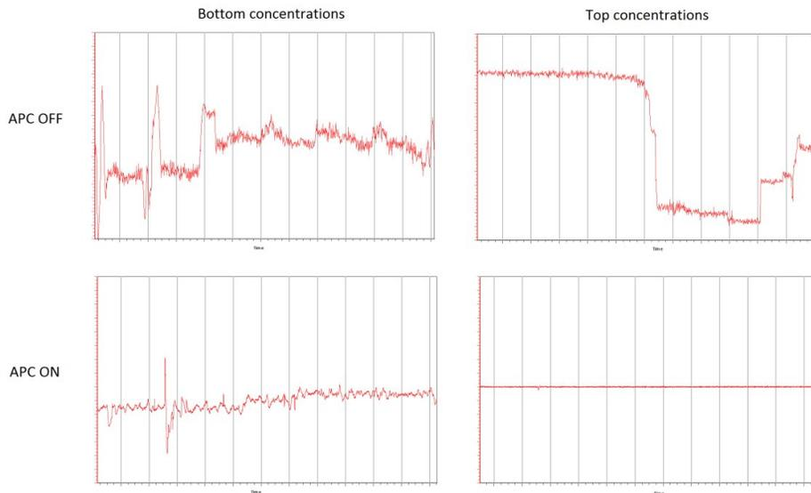
Figure 1: Bottom (left) and top concentration (right) trends over time. Upper plots: APC is turned off. Bottom plots: APC is turned on.
