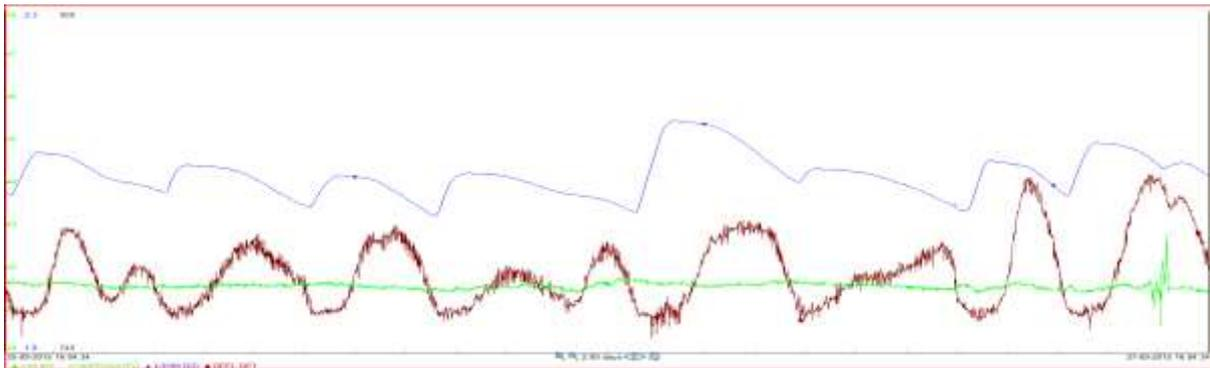
Figure 3: New APC control with modified reflux ratio control for top temperature
