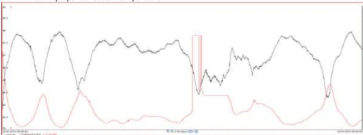
Figure 4: Disturbance in bottom temperature due to over-refluxing and analyser goes off-range
