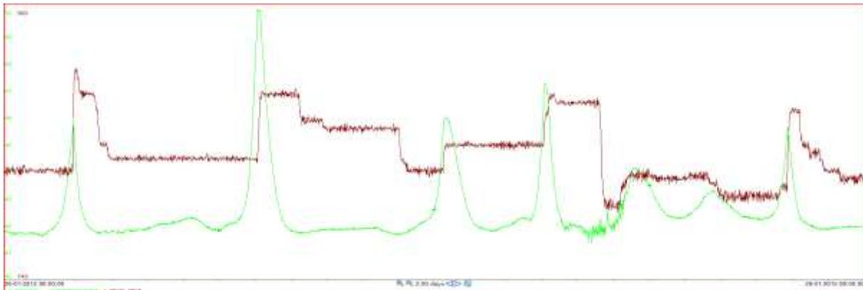
Figure 2: Before trends for the top temperature with APC OFF due to the cyclic disturbances
