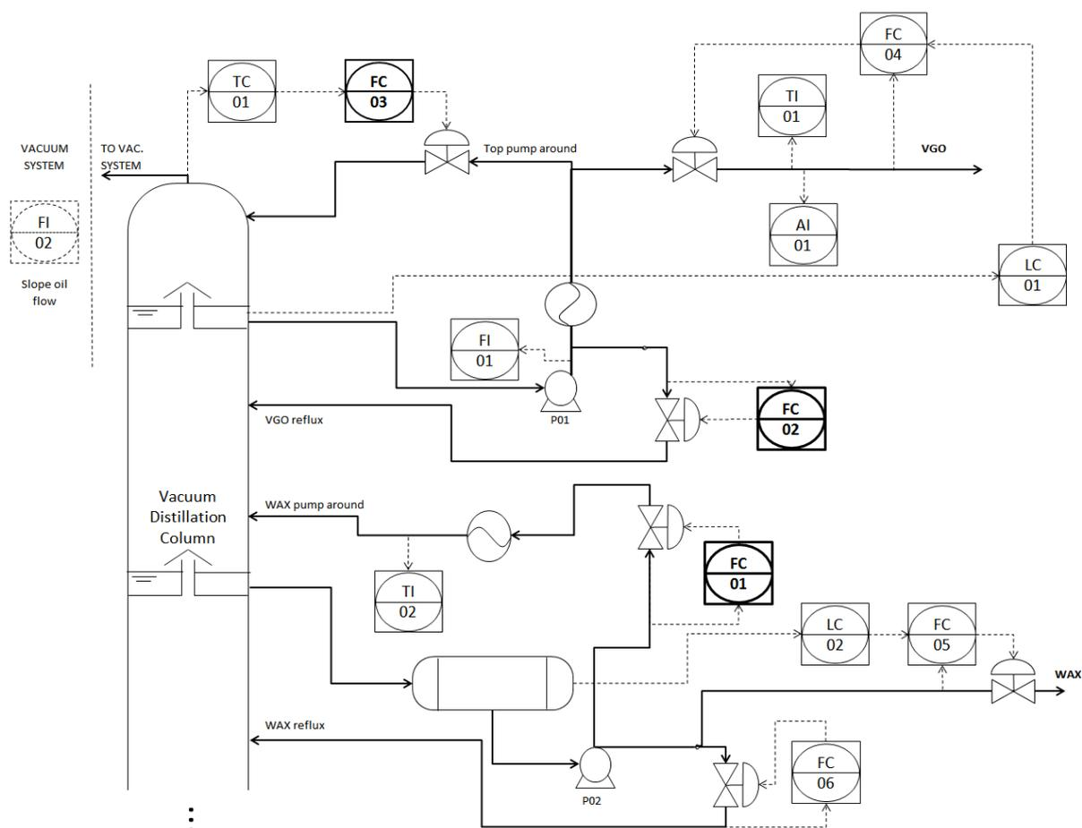
Figure 1 – Vacuum distillation column top section control scheme
