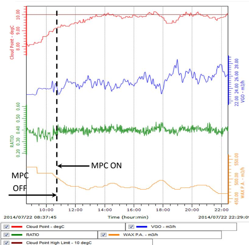
Figure 5 – VGO production maximization while keeping cloud point within specification (1)
