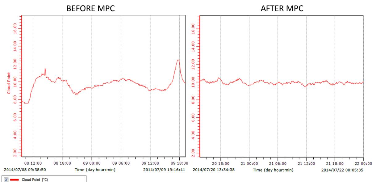
Figure 3 – VGO cloud point stabilization
