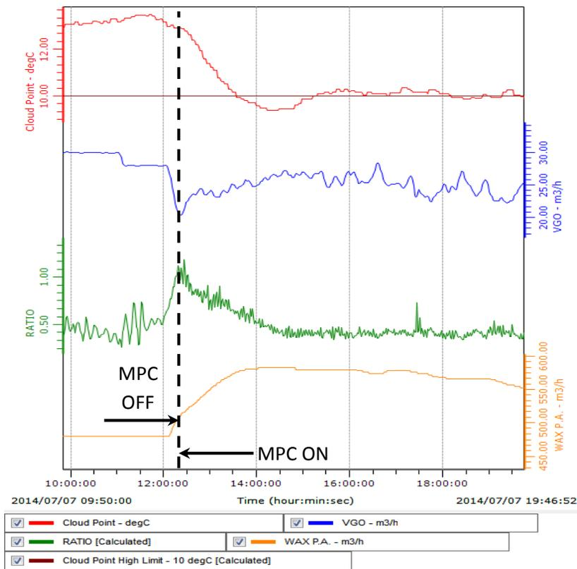
Figure 4 – VGO cloud point brought back to specification after turning MPC ON
