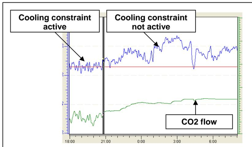
Figure 5: Maximizing throughput until a constraint is active
