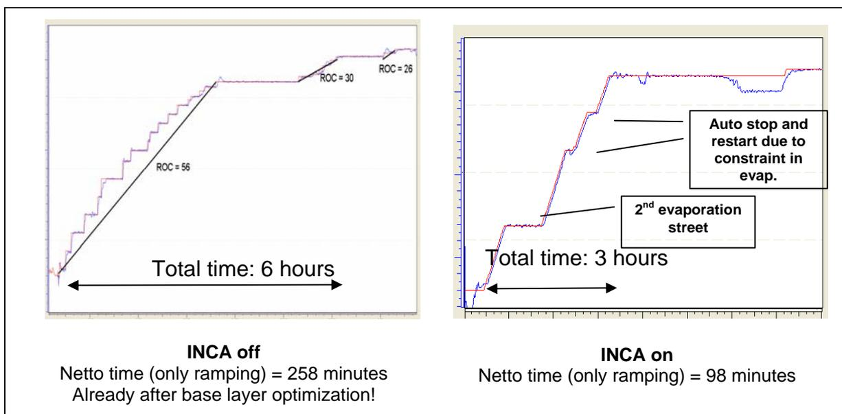
Figure 7: Ramping of CO<sub>2</sub> flow from 50% to 100% load with INCA turned off (l) and INCA turned on (r)
