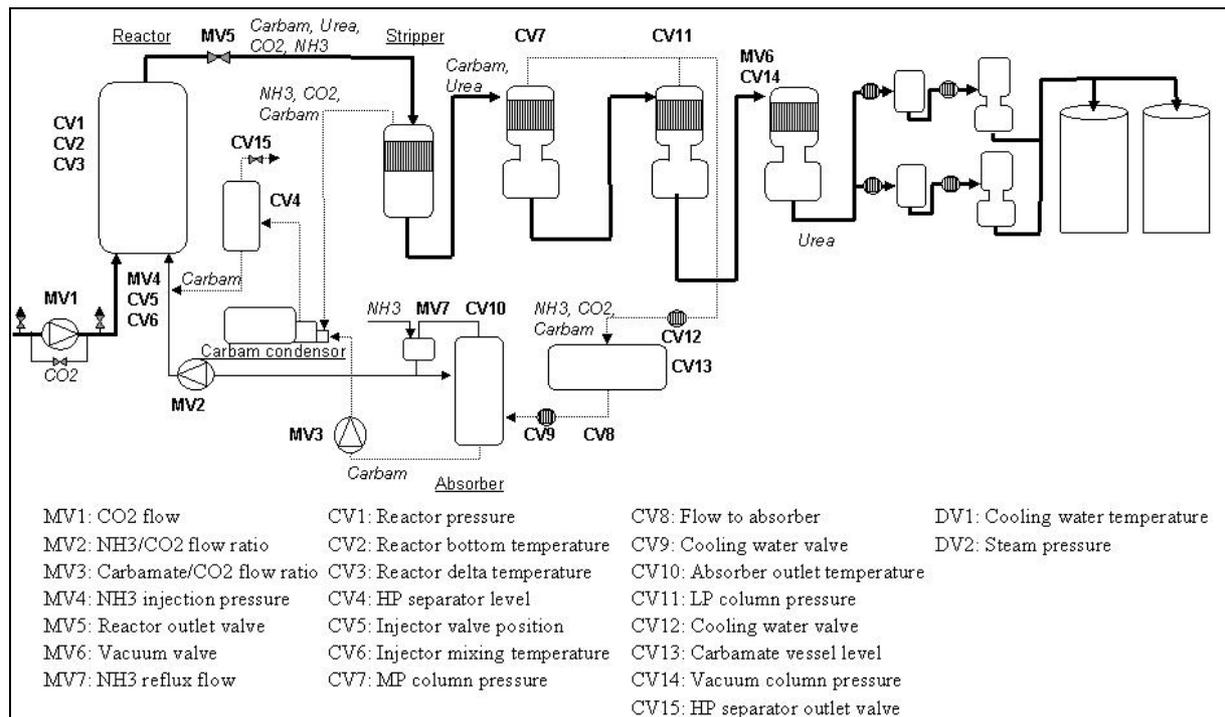
Figure 1: Schematic overview of a urea plant with INCA model variables
