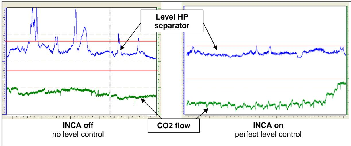
Figure 4: HP separator level with INCA turned off (l) and INCA turned on (r)
