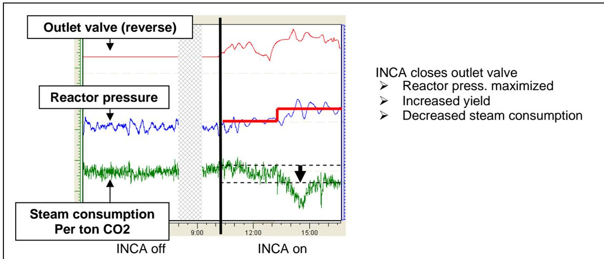
Figure 6: Increased yield by turning on INCA. Closing the outlet valve causes the reactor pressure and the yield to increase.
