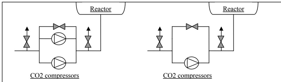
Figure 3: CO<sub>2</sub> compressors at 100% load (left) and at 50% load (right)
