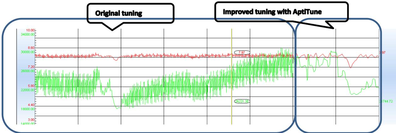
Legend: In the plot above the Red line represents the Drum pressure PV; The green is the fuel gas flow from the coker drum.
