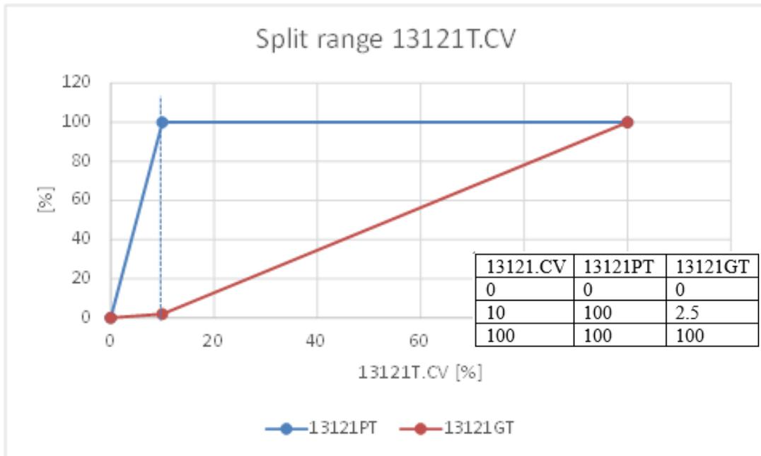
Figure 5 – Transformation 13121PT and 13121GT in function of 13121T.CV
