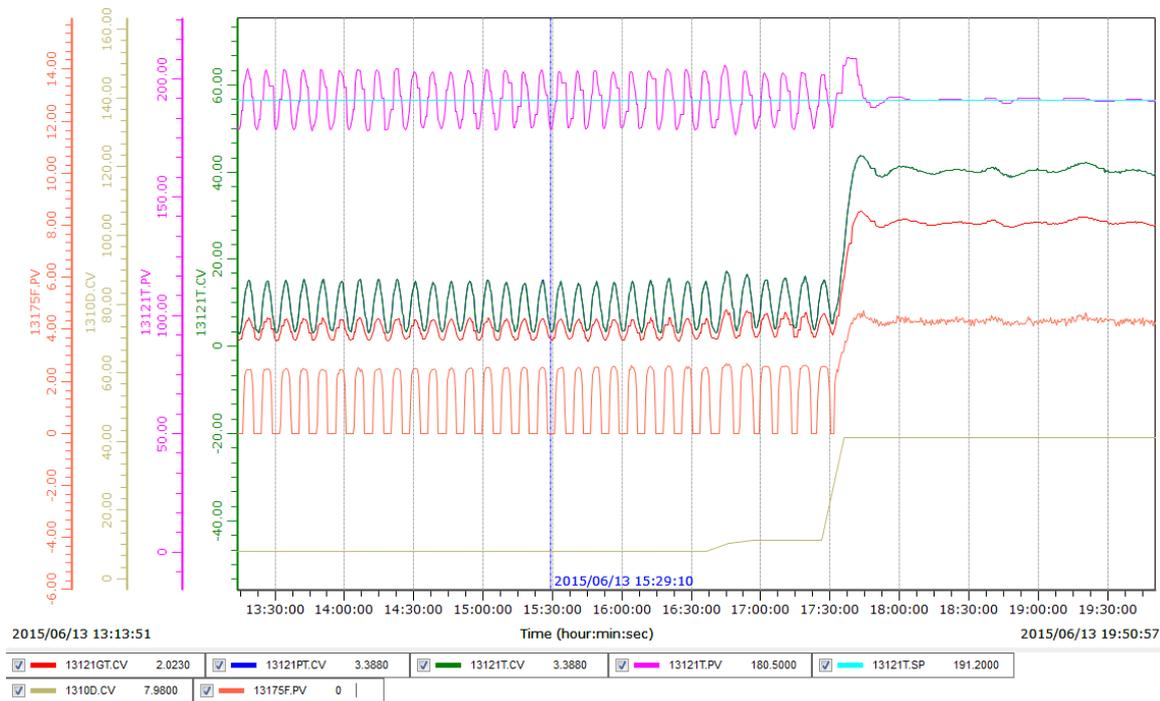
Figure 2 - Initial performance temperature controller 13121-TC
