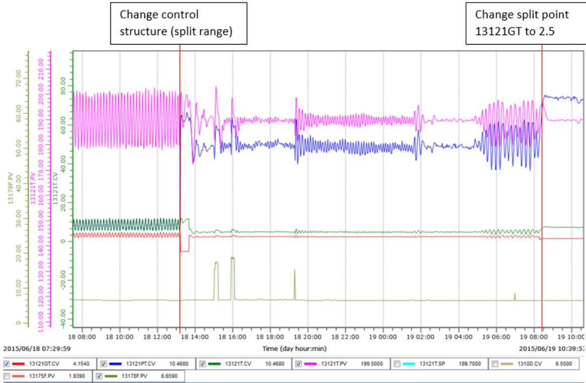
Figure 6 - Controller performance before and after implementation of split range control
