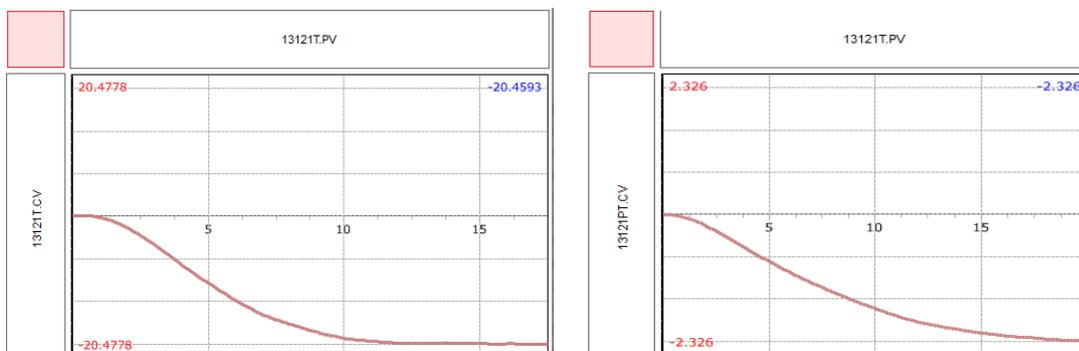
**Figure 4 - Relative gain of the 13121GT (left) and 13121PT (right) to the temperature 13121T**
