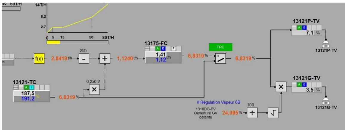
Figure 1 - DCS control scheme temperature control 13121-TC
