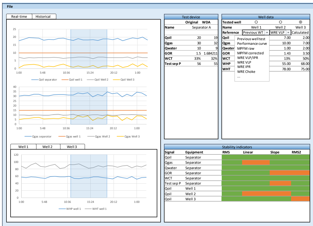
FIGURE 2 VIRTUAL METERING BASED TEST BY DIFFERENCE
